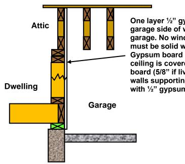
One layer  $\frac{1}{2}$ " gypsum board applied on garage side of wall between house and garage. No windows. Doors to dwelling must be solid wood or metal. Alt. Gypsum board may stop at ceiling if ceiling is covered with  $\frac{1}{2}$ " gypsum board (5/8" if living space above) and walls supporting the ceiling are covered with  $\frac{1}{2}$ " gypsum board.
