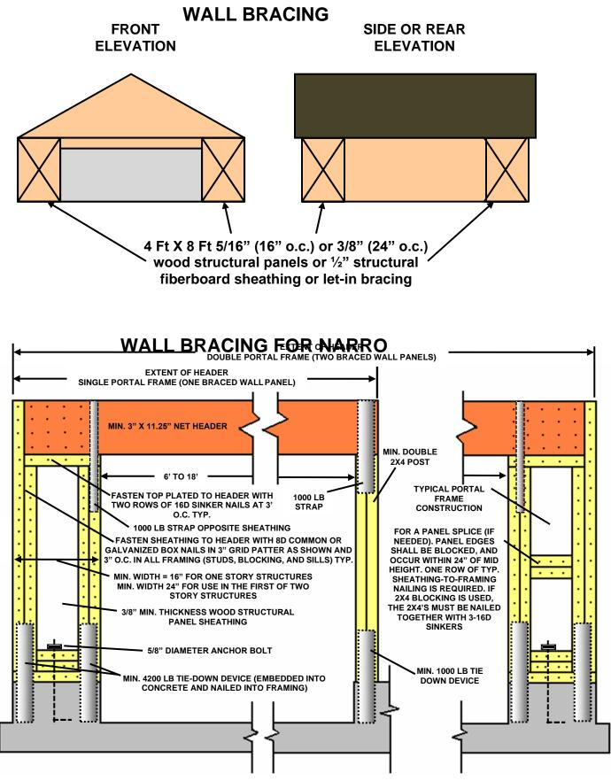
ALTERNATE BRACED WALL PANEL ADJACENT TO A DOOR OR WINDOW OPENING
